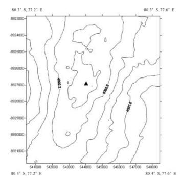
**Fig. 1.** Dome A surface topographic map based on GPS data from the 21st CHINARE. Heights are relative to the WGS84 ellipsoid. Contour interval is 0.40 m. The black triangle indicates the position of the summit of Dome A.
