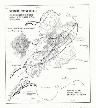
Fig.4. Predicted location of watersheds and ice divides on western Vatnajökull, drawn on a map showing the bedrock topography (Björnsson in press). The basins drain melt water to the rivers Tungnaá, Sylgja and Kaldakvisl. The ice cauldrons drain water to Skaftá.
