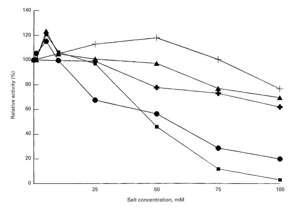
**Fig. 1.** Effects of NaCl (+), KCl ( $\bullet$ ), sodium citrate ( $\blacksquare$ ), NH<sub>4</sub>Cl ( $\blacktriangle$ ) and K<sub>2</sub>SO<sub>4</sub> ( $\bullet$ ) on the activity of purified buffalo-milk lysozyme (3 milliunits in 3 ml reaction mixture). Values are means of 3 determinations expressed as percent activity.
