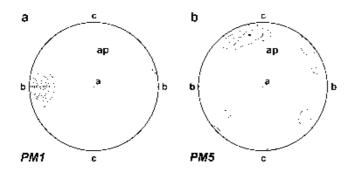
**Fig. 5.** Fabric diagrams of ice-wedge ice: (a) sample PM1, 36 crystals; (b) sample PM5, 39 crystals. Diagrams in vertical plane parallel to axial plane. a is normal-direction ice at wedge centre, b is parallel-direction ice at wedge boundary, c is vertical direction and ap is axial plain. Fabric diagrams are plotted as lower-hemisphere projections on a Schmidt equal-area net. Contours at intervals of 5%, 15%, 25%, 35%, 45%, 55%.
