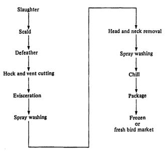
Fig. 1. Outline of stages in a typical poultry processing plant (McMeekin & Thomas, 1979).
