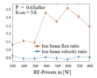
FIGURE 13. Centre ion beam velocity ratio  $v_{Br}$  and ion beam flux ratio  $\phi_{Br}$  versus RF-power at pressure  $P = 0.65 \mu \text{Bar}$  and magnetic coil current  $I_{\text{Coils}} = 5 \text{ A}$ .
