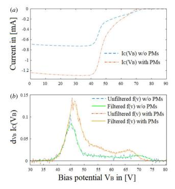
FIGURE 6. (a) Collected current  $I_C$  and (b) unfiltered and filtered distribution functions for an ion beam at RF-power 400 W, pressure  $P = 0.65 \mu$ Bar and coil current  $I_{\text{Coils}} = 5$  A, with and without PMs.
