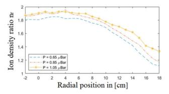
FIGURE 10. Radial ion density ratio versus pressure values  $P = 0.65 \ \mu\text{Bar}$  at flow  $Q = 2.0 \ \text{SCCM}$ ,  $P = 0.85 \ \mu\text{Bar}$  at flow  $Q = 3.0 \ \text{SCCM}$  and  $P = 1.05 \ \mu\text{Bar}$  at flow  $Q = 4.0 \ \text{SCCM}$  at RF-power 400 W and magnetic coil current  $I_{\text{Coils}} = 5 \ \text{A}$ .
