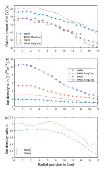
FIGURE 8. Radial profiles of (a) the plasma potential  $V_p$ , (b) the ion density  $n_i$  and (c) ion density ratio  $n_r$  versus RF-power at pressure  $P = 0.65 \mu$ Bar and magnetic coil current  $I_{\text{Coils}} = 5$  A at RF-power 400 and 800 W, with and without the magnet band.
