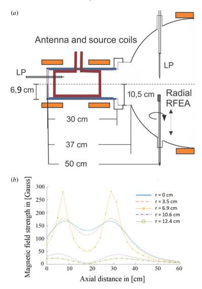
FIGURE 1. (a) An overview of the Njord device and its dimensions and (b) a simulation of the axial magnetic field strength induced by the coils at different radial values at coil current  $I_{\text{Coils}} = 5$  A, which includes the centre, the outer radius of the Pyrex tube (r = 6.9 cm), the inlet chamber (r = 10.5 cm) and at the position of the coils (r = 12.4 cm).
