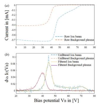
FIGURE 5. (a) Raw data from the collected current  $I_C$  and (b) raw versus filtered distribution function for an ion beam and background plasma at 400 W,  $P = 0.65 \mu$ Bar and  $I_{\text{Coils}} = 5$  A, without PMs.
