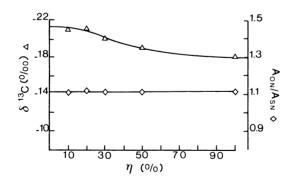
Fig 4. Mortar from Heilige-Kruis Church at Vrasene (Belgium). Very pure sample from lime slaking, hardly any trace of fossil carbonate present.  $^{14}$ C dating confirmed that the sample came from 12th and not 14th century construction.
