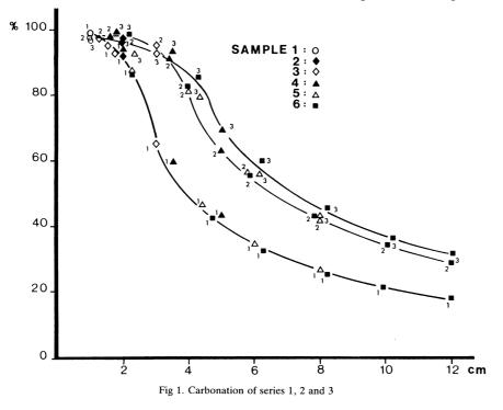
of  $CO_2$  starts at the surface and ends at the point indicated on the abscissa (1st, 2nd & 3rd series). Figure 1 shows that the total height of the pillar has no influence on the carbonate content of a certain level. Only the
