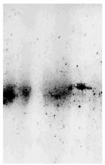
Fig. 5. A negative image taken in the geometry of Figure 4. Here the laser light is across the image from right to left, and the dark band across the center represents light scattered by dust. Other black spots are due to bubbles in the ice; they are large and very efficient scatterers of even stray light. Note the abruptness of the dusty-to-clear transition.
