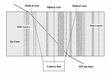
Fig. 3. A cartoon of an ice core with dusty layers with oblique laser illumination and a camera to record scattered light.
