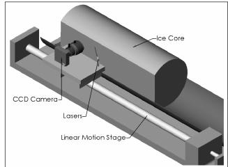
Fig. 4. As in Figure 3 except a computer-aided drawing of the observational system for using oblique laser scattering with an ice core. The core has a flat on one side as is usual for modern cores.
