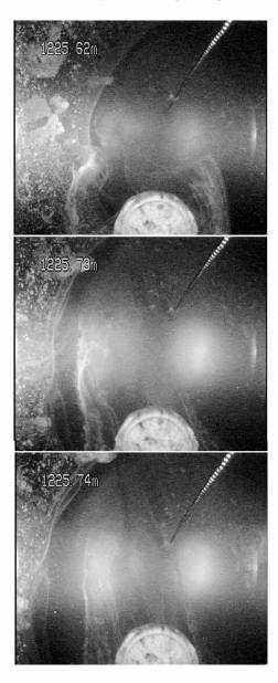
Fig. 1. Down-looking images from the IBC deployed at 1225 m in Ice Stream C, Antarctica. A chain, as an aid to determining depth of viewing, and a compass, out of focus in this picture, are visible, as is the borehole wall. This kind of image is designed to provide data on bed nature and relative movement.
