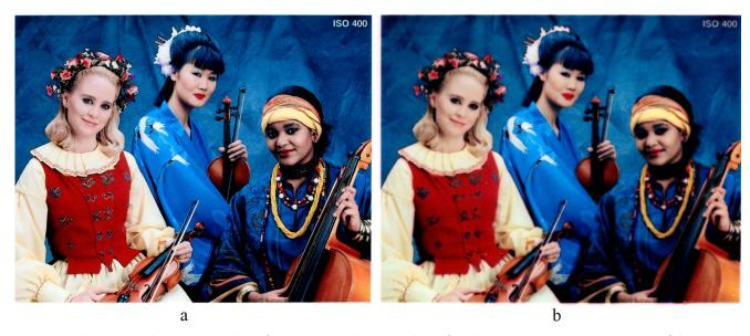
FIGURE 5. Inkjet prints showing examples of (a) the original print and (b) after dye migration. Images courtesy of the Image Permanence Institute.
