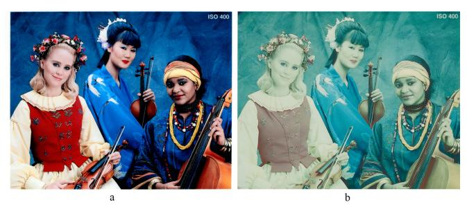
FIGURE 4. Inkjet prints showing examples of (a) the original print and (b) after fading and hue shift. Images courtesy of the Image Permanence Institute.
