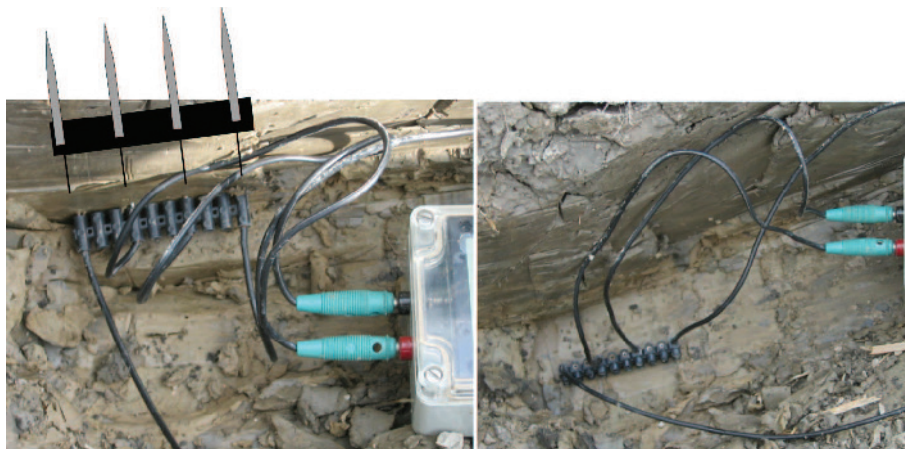
Figure 13. Photographs of parallel and perpendicular ER measurements using SSM1.
