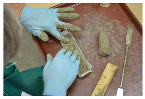
**FIGURE 3.** Pressing a "log" of plastic sample clay into a test bar template, lined with parchment paper (our template is recycled from an old army surplus industrial dishwasher rack; soon we will have a printable 3D file of this template to share with interested researchers).
