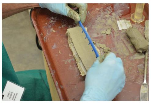
**FIGURE 4.** Marking scoring distances on sample clay test bar (with recycled hair comb tool). Take care that follow-up scoring lines are shallow (about 1 mm) to avoid compromising the integrity of the bar (if too deep, the bar may separate along a scored line during drying).
