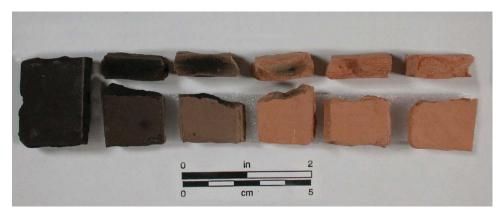
FIGURE 8. Fired briquettes are broken to record color change and coring loss.
