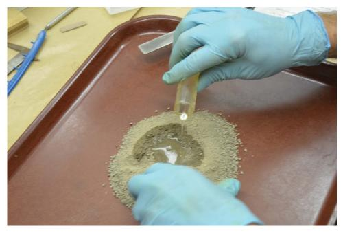
FIGURE 1. Water is added to depression in the pile of dry, crushed clay sample.
