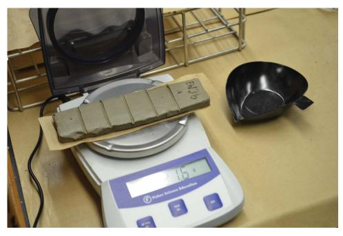
FIGURE 6. Weighing completed sample clay test bar for wet weight used in calculating percent Water of Plasticity.
