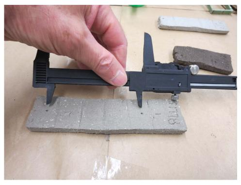
FIGURE 5. Marking bar with 10-cm distance with metric calipers for percent Linear Drying Shrinkage measurement.
