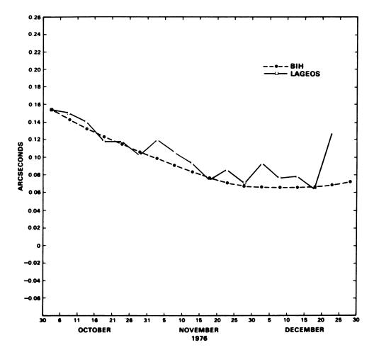
Figure 2. Y-component of polar motion.
