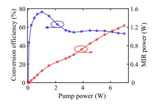
**Figure 4.** Generated mid-infrared power and corresponding conversion efficiency vary as functions of the pump power. Note that the conversion efficiency was defined as total power of down-converted fields divided by the initial pump power. Connecting lines are only used to guide the eye.
