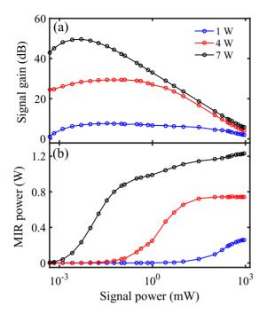
**Figure 5.** (a) Signal gain against input signal power for different pump power. (b) Generated MIR power versus injected signal power under various settings of pump power. Solid lines are used to guide the eyes only.
