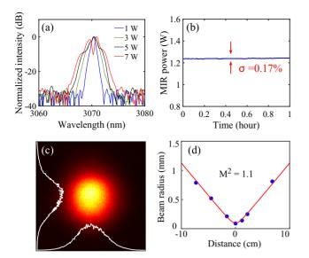
**Figure 3.** (a) MIR spectra under different pump power. The signal power was kept at 900 mW. (b) Power stability of the mid-infrared output.  $\sigma$  indicates the relative fluctuation. (c) MIR beam image at the near field as well as two section profiles along orthogonal axes. (d) Evolution of MIR beam waists along the propagation distance. Note that the central position was defined at the focal point.
