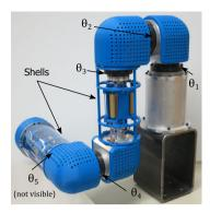
*Figure 2.* Photograph of the experimental 5-DOF robot with the low-impedance displacement sensors mounted on links 3 and 5, figure taken from [23].
