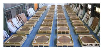
**Figure 4.** Crearceram glass ceramics blanks are in full production for TMT's primary mirror in Japan. These 1.52-m circular discs go through stages of grinding, aspherical polishing, hexing, mounting before going overseas for final touch up, and eventually to the telescope site. TMT needs 594 of such segments. This is another example of utilizing what is available in the industry to specialize to match the research needs.
