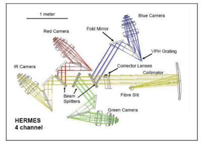
Figure 1. Optical design of the HERMES four-band high-resolution spectrograph.
