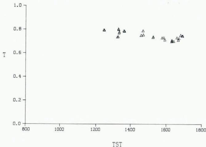
Fig. 4. Radiation transmittance  $T$  as a function of true solar time  $TST$  during ice decay (8 March 1977).
