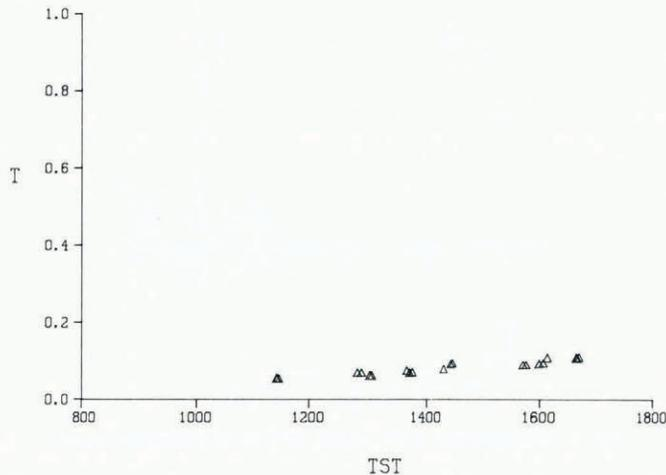
Fig. 2. Increase in radiation transmittance due to snowmelt as indicated by the rise in transmittance ratio  $T$  with true solar time TST (22 February 1977).
