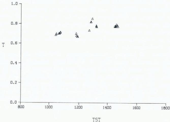
Fig. 3. Ratio of below- to above-ice radiation  $T$  as a function of true solar time  $TST$  during a period of melting snow (7 March 1977).
