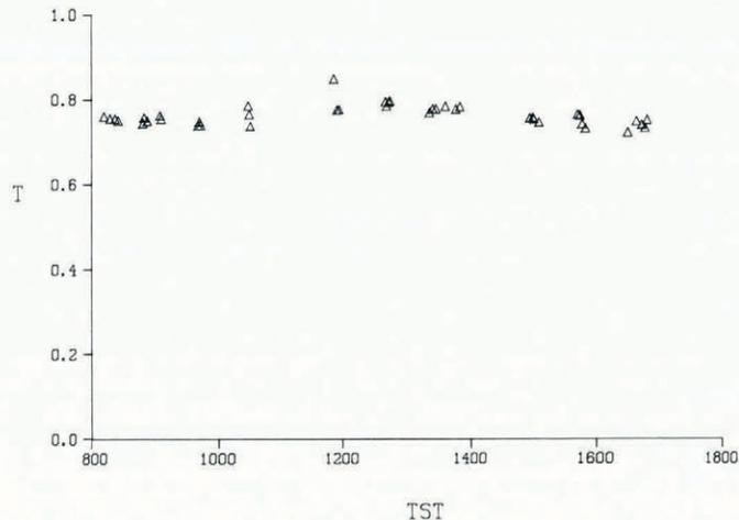
Fig. 5. Radiation transmittance  $T$  as a function of true solar time  $TST$  during ice decay (9 March 1977).
