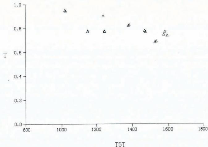
Fig. 6. Transmittance  $T$  versus true solar time  $TST$  showing differences in  $T$  due to cloud-cover variability (18 January 1977)
