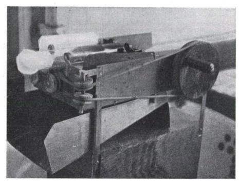
Fig. 1. Hand-driven rolling machine.
