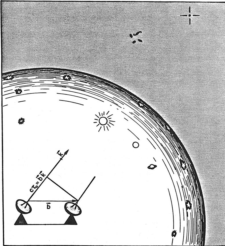
Fig.1 Geometry in a two-element radiointerferometer system
