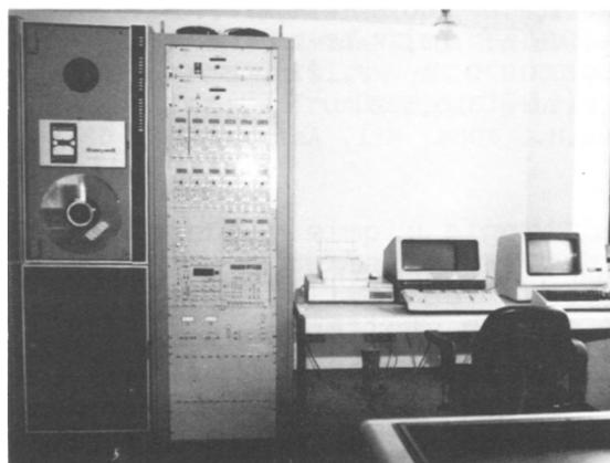
Operators bay with VLBI Mark III DAT magnetic tape unit and HP 1000 terminal
