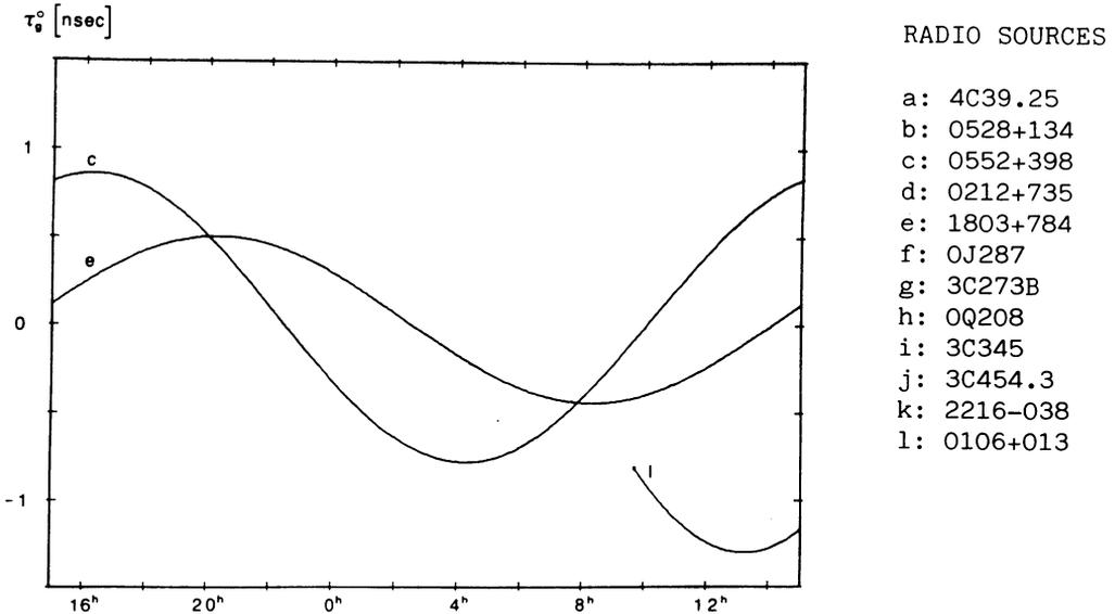
Fig.3 Temporal behaviour of gravitational solar time delay for three selected radio sources for the experiment of Fig.2.
