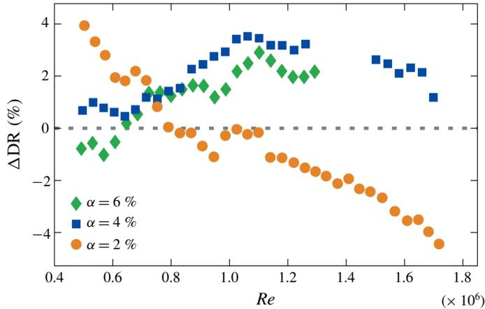
FIGURE 8. Plot of  $\Delta DR = DR_{hydrophobic} - DR_{hydrophilic}$  from figure 7 versus  $Re$ . For  $\alpha = 2$ ,  $\Delta DR$  decreases with increasing  $Re$ , owing to the influence of roughness. For  $\alpha \geq 4$ ,  $\Delta DR$  shows an increase with  $Re$ , meaning that the effect of increase in bubbly drag reduction due the hydrophobic coating is stronger than the effect of roughness.
