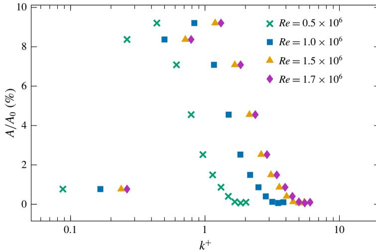
FIGURE 6. Roughness distribution of the surface as coverage fraction of the total area  $A/A_0$ , expressed in wall units for four different values of  $Re$ . Apart from the maximum and the minimum values of  $Re$  used in this research, the normalized roughnesses for two intermediate values of  $Re$  are shown as well. The wall unit normalization is obtained using data from the torque measurements that give an averaged, global value of the wall shear stress.
