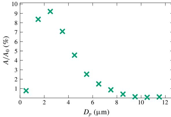
FIGURE 3. Pore size diameter  $D_p$  (roughness) distribution of the coating as a fraction of the coverage  $A$  of the total area of the coating  $A_0$ . A range of length scales are observed, corresponding to the different regions identified in figure 2. The equivalent circle diameter has been used as a measure of the size  $D_p = 2\sqrt{A_p/\pi}$ .
