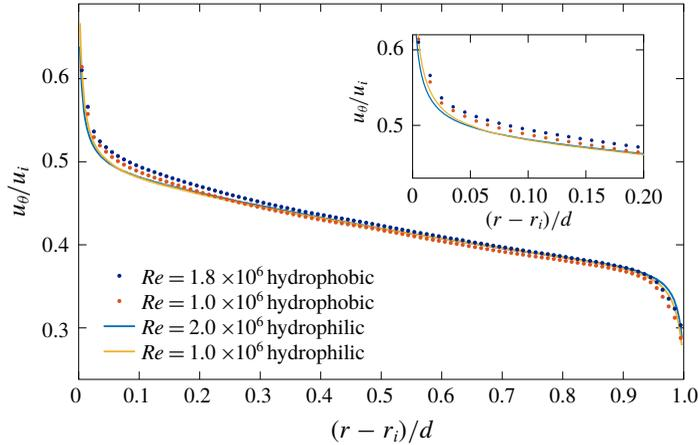
FIGURE 10. Plot of azimuthal velocity normalized with inner cylinder velocity  $u_{\theta}/u_i$  versus the normalized gap width between inner and outer cylinder  $(r - r_i)/d$ . The working fluid is without air, so  $\alpha = 0\%$ . Compared is the rough hydrophobic coating with the smooth hydrophilic steel inner cylinder. The hydrophilic data are provided by Huisman *et al.* (2013) using the same experimental set-up. The inset shows the region close to the inner cylinder.
