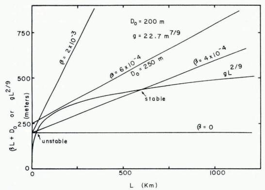
Fig. 4. Plots of the functions  $gL^{2/9}$  and  $(\beta L + D_0)$  versus L. Curves plotted for  $g = 22.7 m^{7/9}$ ,  $D_0 = 200 m$  and (for one curve) 250 m, and  $\beta = 2 \times 10^{-3}$ ,  $6 \times 10^{-4}$ ,  $4 \times 10^{-4}$  and o. Values of L for steady-state ice sheets occur where the curves of  $gL^{2/9}$  and  $(\beta L + D_0)$  cross.
