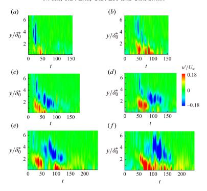
Figure 5. Evolution of the streamwise fluctuating velocity of turbulent spots in the y-t plane: (a)  $x/\delta_0^* = 25$  in Domain 1; (b)  $x/\delta_0^* = 45$  in Domain 1; (c)  $x/\delta_0^* = 55$  in Domain 2; (d)  $x/\delta_0^* = 75$  in Domain 2; (e)  $x/\delta_0^* = 115$  in Domain 3; (f)  $x/\delta_0^* = 135$  in Domain 3.
