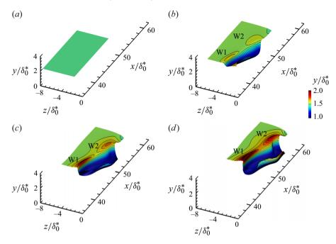
Figure 23. Development of a material surface initiated at  $y/\delta_0^* = 1.5$  and t = 76 in the low-speed region labelled I in figure 19: (a) t = 76; (b) t = 82; (c) t = 88; (d) t = 94.
