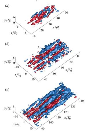
Figure 6. Evolution of the isosurfaces of streamwise fluctuating velocity in the experiment: (a) Domain 1; (b) Domain 2; (c) Domain 3. The blue and red isosurfaces correspond to the negative and positive streamwise fluctuating velocities, respectively. The isosurfaces in panel (a-c) correspond to  $u'/U_{\infty} = \pm 6.5$  %. There is no time correlation among panels (a), (b) and (c).
