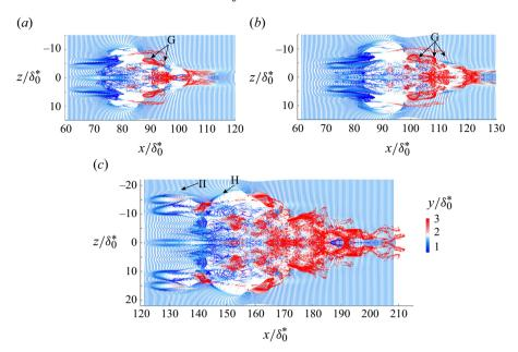
Figure 20. Timelines of the turbulent spot at a sequence of stages: (a) t = 156; (b) t = 176; (c) t = 276. The timelines in panels (a) and (b) are initiated at t = 36,  $x/\delta_0^* = 61$  and  $y/\delta_0^* = 1.2$ . The timelines in panel (c) are initiated at t = 86,  $x/\delta_0^* = 121$  and  $y/\delta_0^* = 1.2$ .
