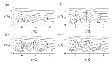
Figure 14. The y-z plane cross-sections of material surfaces initiated at a series of heights and t = 86.4: (a)  $x/\delta_0^* = 112$  and t = 92.6; (b)  $x/\delta_0^* = 114$  and t = 95.7; (c)  $x/\delta_0^* = 116$  and t = 98.8; (d)  $x/\delta_0^* = 118$  and t = 101.9.
