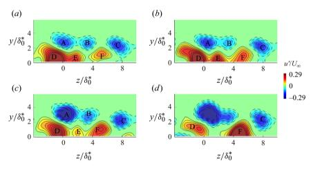
Figure 15. Contours of streamwise fluctuating velocity displaying the amalgamation of the low-speed streaks: (a)  $x/\delta_0^* = 112$  and t = 92.6; (b)  $x/\delta_0^* = 114$  and t = 95.7; (c)  $x/\delta_0^* = 116$  and t = 98.8; (d)  $x/\delta_0^* = 118$  and t = 101.9.
