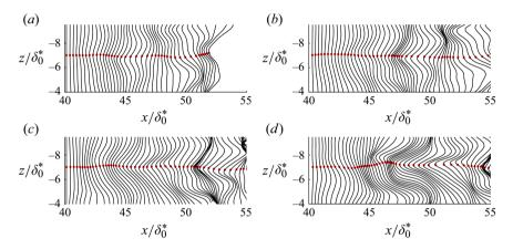
Figure 9. Evolution of spanwise timelines initiated at  $x/\delta_0^* = 41$ ,  $y/\delta_0^* = 1.1$  and t = 24.7 showing the low-speed streak labelled A in figure 6(b): (a) t = 30.9; (b) t = 38.6; (c) t = 46.3; (d) t = 54.0. The sequence of red dots corresponds to a streakline initiated at  $z/\delta_0^* = 7$ .
