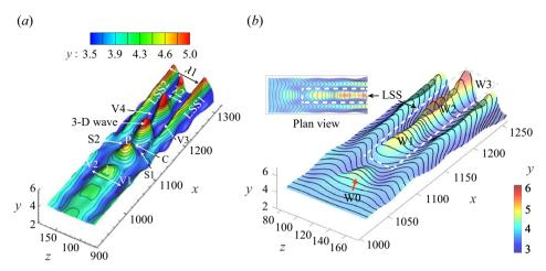
Figure 1. Wave-like behaviour of low-speed streaks in the O-type transition boundary layers: (a) material surface of Jiang et al. (2020a) (used with permission); (b) spanwise timelines of Jiang et al. (2020b) (used with permission).
