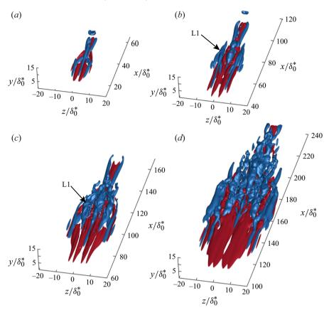
Figure 18. Development of the isosurfaces of streamwise fluctuating velocity for DNS: (a) t=76; (b) t=136; (c) t=196; (d) t=296. The blue and red isosurfaces correspond to the streamwise fluctuating velocity at  $u'/U_{\infty}=-10$ % and  $u'/U_{\infty}=10$ %, respectively, where  $U_{\infty}$  is the free stream velocity.
