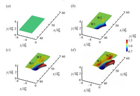
Figure 24. Development of a material surface initiated at  $y/\delta_0^* = 1.0$  and t = 76 in the low-speed region labelled I in figure 19: (a) t = 76; (b) t = 82; (c) t = 88; (d) t = 94.
