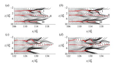
Figure 12. Spanwise timelines showing the low-speed streaks within the turbulent spot in Domain 3. (a,b) Spanwise timelines initiated at  $x/\delta_0^* = 106.3$ ,  $y/\delta_0^* = 1.6$  and t = 74.1. (c,d) Spanwise timelines initiated at  $x/\delta_0^* = 122.1$ ,  $y/\delta_0^* = 1.6$  and t = 95.7. The sequences of the red particles are streaklines initiated at  $z/\delta_0^* = 0.4$ , 3.2, and 7.9: (a) t = 92.6; (b) t = 95.7; (c) t = 114.2; (d) t = 117.3.
