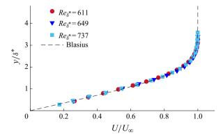
Figure 3. Comparison between the measured velocity profiles and Blasius profile.
