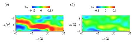
Figure 10. Vorticity colour maps in the x-z plane at  $y/\delta_0^* = 1.1$  and t = 54: (a) wall-normal vorticity  $\omega_y$ ; (b) streamwise vorticity  $\omega_x$ .
