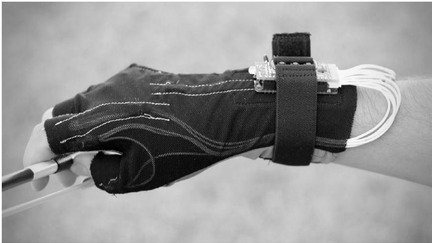
**Figure 3.** Alto.glove, a wireless sensor glove for violin developed by the author.
