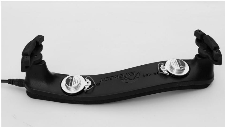
**Figure 2.** A modified violin shoulder rest with embedded voice coils developed by the author.
