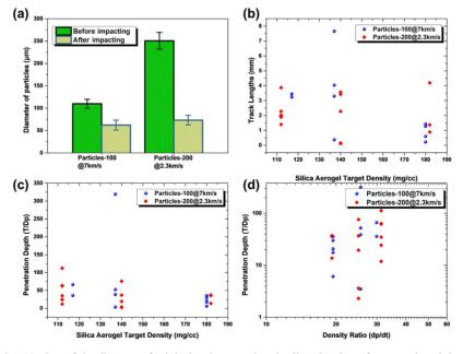
**Figure 6.** Summary of results: (a) plots of the diameter of original and captured projectiles; (b) plots of measured track lengths shown as a function of aerogel target density, all at 2.3 and 7 km/s by impacting (measurement error is  $\pm 0.002$  mm); (c) the aerogel track lengths (*T*) normalized to projectile diameter ( $D_p$ ) against target bulk density; (d) penetration track length scaled ( $T/D_p$ ) against density ratio ( $d_p/d_t$ ).
