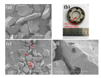
Figure 1. SEM images of irregularly shaped  $Al_2O_3$  grains of (a) Particles-100 and (c), (d) Particles-200 (with surface holes) used as projectiles in the PG experiment. (b)  $Al_2O_3$  grains on Mylar film.
