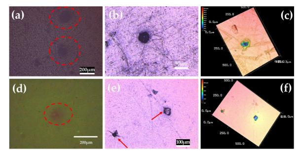
Figure 4. Observation of the track entrance: (a) attachments of Mylar near the track entrance marked by red circles: (b) near circular entrance hole of a penetration track; (c), (e), (f) irregular shape of penetration entrance hole; (d) unclear observation of entrance by VMM; (f) three-dimensional graph matching with (e).
