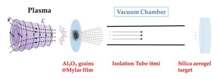
Figure 2. Schematic diagram of projectile flight in the PG.
