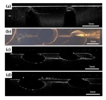
**Figure 10.** Aerogel tracks created by impacts of  $Al_2O_3$  at 7 km/s (the impact direction is from the right). (a) A track-scan photograph along the impact direction. (b) The track photograph just passing through the two spherical bubbles near the cylindrical aerogel side obtained by VMM. (c), (d) The two segments of the track of (b) revealed by OCT.
