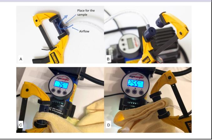
Filtration performance index of each tested fabric was defined as the area under the fitted curve (AUC) of filtration efficiency versus airflow resistance percentage of the highest N95 mask resistance recorded (15.5 psi).
