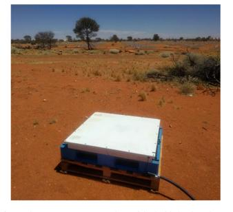
Figure 9. The prototype SKAPA cosmic ray detector (white box) deployed near the MWA core at the MRO. It is raised off the ground with palettes to avoid surface water. Power and data return are enclosed via the black cable housing. The detector has been tested to ensure compliance with MRO RFI requirements and has been detecting cosmic ray muons since its deployment in October 2018. *Photo credit*: Justin Bray.
