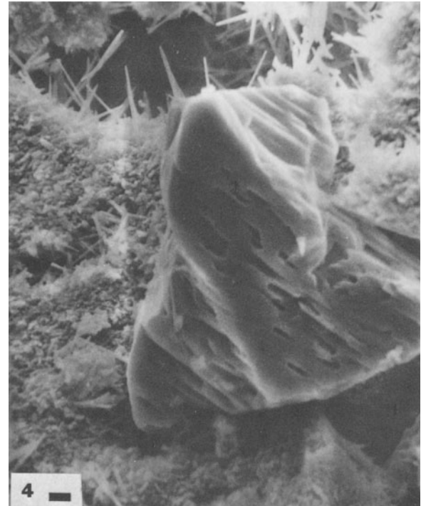
Fig. 1. Kaolinite in quartz geode from Mississippian Warsaw shale, near Keokuk, Iowa, 1500 \times . Scale is one (1) micrometer unless otherwise designated.
