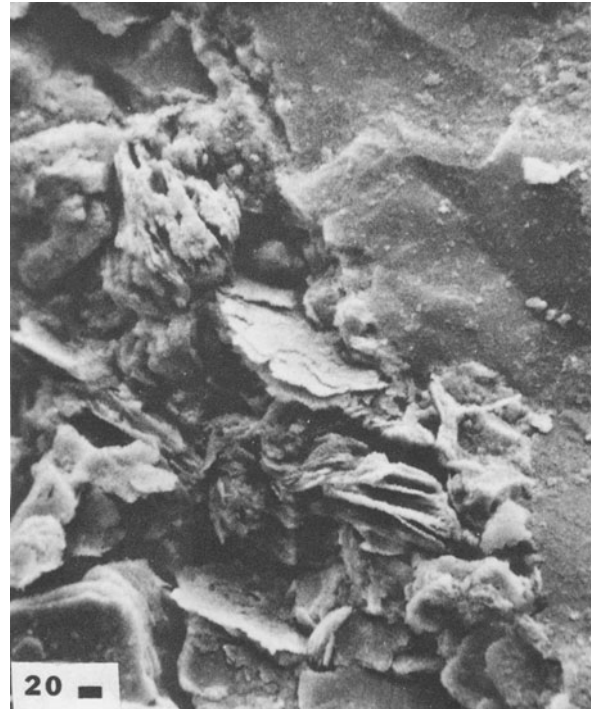
Fig. 17. Kaolin in the residual deposit at Caminau, near Bautzen, East Germany, GDR, 5000 \times .
