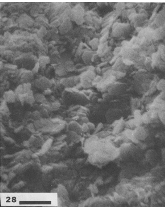
Fig. 25. Kaolin from drill core penetrating alteration zone of granite, Blackpool Pit, Cornwall District, 4000 \times .
