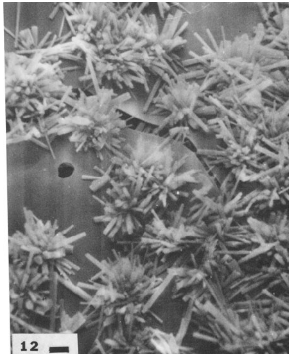
Fig. 9. Kaolin on feldspar in gneiss, 25 km south of Athens, Ga. 4000 \times .
