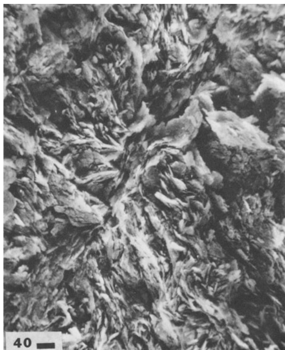
Fig. 37. "Hard" kaolin, API Reference Clay, Dixie Pit, Bath, S.C., 5000 \times .
