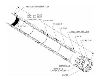
Fig. 1. Core barrel and cutter head.
