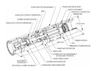
Fig. 3. Motor section.
