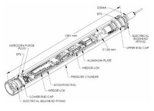
Fig. 5. Instrument section.
