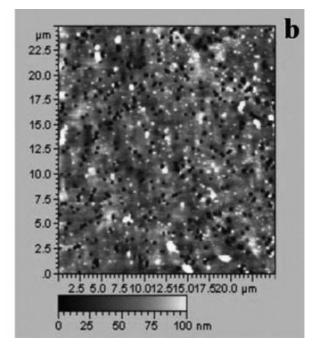
Fig. 1. Atomic Force Microscopy images (25×25 μm) of a 0.4 μm polycarbonate filter before (a) and after (b) sampling.
