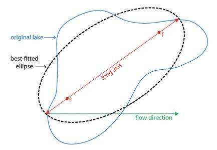
**Fig. 1.** Schematic of optimal fit of an ellipse (with f indicating the foci) to the outline of a previously identified lake. The ellipse and original lake are equal in area. The angle between the long axis of the ellipse and the flow direction (either clockwise or anticlockwise) determines the ellipse orientation.
