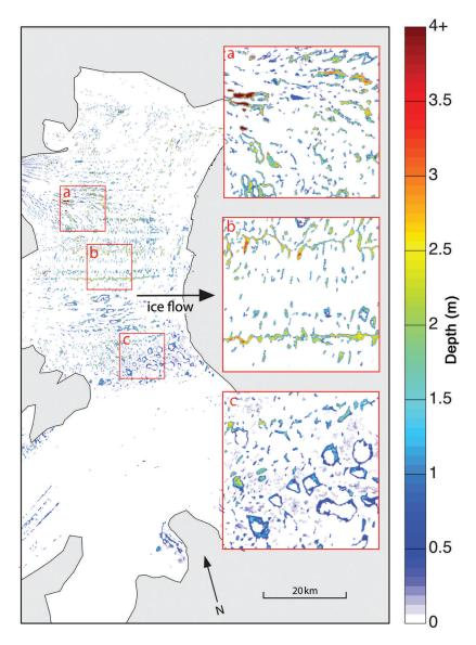
**Fig. 2.** Depths of lakes on the Larsen B ice shelf using reflectance of the 21 February 2000 Landsat image. Although some lake depths are >4 m, for visualization purposes 4 m is plotted as the maximum depth here. Three areas, a, b and c, are enlarged to show varying lake characteristics and patterns across the ice-shelf surface. Marginal areas, which can be grounded ice, bare land surface or ocean surface, are shaded grey.
