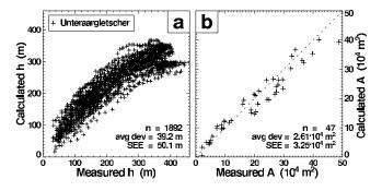
**Fig. 5.** Comparison of calculated and measured ice thickness h (a) and cross-sectional area A (b) for Unteraargletscher (n: number of points; avg dev: average deviation; SEE: standard error of estimate).
