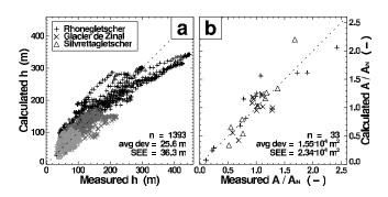
**Fig. 4.** Comparison of calculated and measured (a) ice thickness h and (b) cross-sectional area A. For better visualization, the cross-sectional area is normalized with the mean measured area  $A_N$ . The statistics, bottom right, refer to the whole ensemble of points (n: number of points; avg dev: average deviation; SEE: standard error of estimate).
