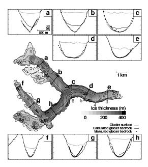
**Fig. 9.** Calculated and measured ice-thickness distribution of Unteraargletscher. The insets (a–h) show the marked cross-sections. All have the same vertical exaggeration. ice-flow velocity measurements are available for the grey dashed profiles with numbers.
