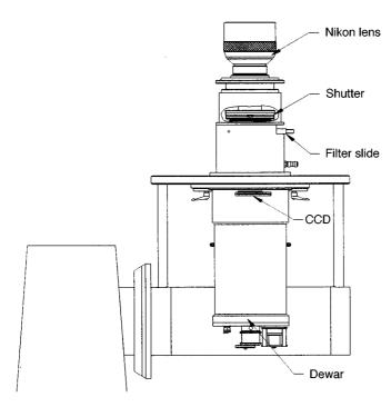
Figure 1—Wide-field camera and CCD as set up at the 16 inch telescope, at Siding Spring Observatory.
