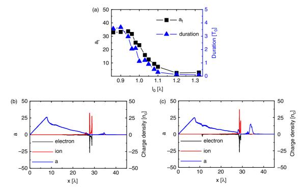
**Figure 3.** (a) Amplitude peak  $a_t$  (black square) and duration (blue triangle) of transmitted pulses versus foil thickness  $t_0$ . For the incident laser,  $a_0/t_{\rm up}=7.35$  ( $a_0=30$  and  $t_{\rm up}=4.08T_0$ ). The foil density is  $n_0=8n_c$ . Laser profile (blue solid line) and charge density of electrons (black solid line) and ions (red solid line) for  $a_0/t_{\rm up}=7.35$  ( $a_0=40.4$  and  $t_{\rm up}=5.5T_0$ ) and (b)  $t_0=1.32\lambda$ , (c)  $t_0=1.32\lambda$ .
