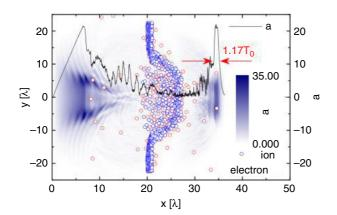
**Figure 5.** Electron (red circle) and ion (blue circle) distribution and the laser profiles in the (x, y) plane for foils with  $n_0 = 8n_c$  and  $l_0 = 1.03$  irradiated by CP laser pulses with  $a_0/t_{\rm up} = 7.35$  ( $a_0 = 30$  and  $t_{\rm up} = 4.08T_0$ ) at  $t = 40T_0$ . The axial laser profiles at y = 0 are denoted by the black solid lines
