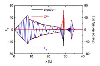
**Figure 4.** Laser profile  $E_{\gamma}$  (blue solid line) and charge density of electrons (black solid line) and  $C^{6+}$  ions (red solid line) for  $a_0/t_{\rm up}=15$  ( $a_0=80$  and  $t_{\rm up}=6T_0$ ). The foil density is  $n_0=15n_c$ , and the foil thickness is  $l_0=1.25\lambda$ .
