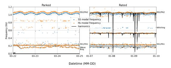
*Figure 2.* SS (blue) and FA (orange) detected modes through automated OMA for both the parked (left) and rated (right) operational conditions, highlighting the interference of rotor harmonics for SS2 and FA2.
