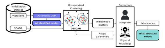
*Figure 4.* Flowchart illustrating the construction of the initial physical modes used for training the normalization and tracking models, as shown in Figure 5.
