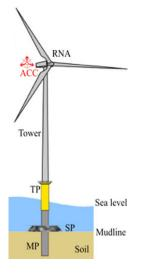
Figure 1. Monopile-supported OWT monitoring setup with one ACC at tower top.
