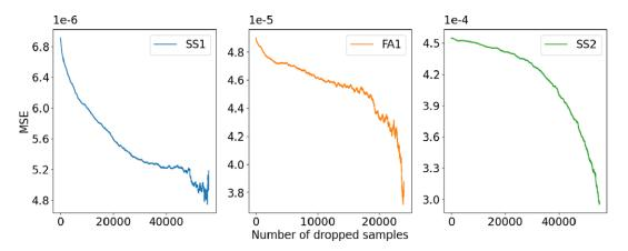
*Figure 7.* Sparsification error curves for the physical modes of an OWT, obtained by sequentially removing the most uncertain predictions and showing the effect on the model performance through MSE.
