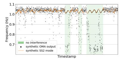
*Figure 10.* Creation process of the synthetic dataset, with the synthetic SS2 mode created through an LR (orange) and the synthetic OMA output generated by overlaying the 6P harmonic (black), showing periods with and without (green) interference.
