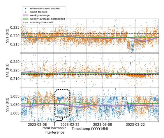
**Figure 9.** Control charts for monitoring the OWT natural frequencies after weekly data averaging (purple), using the reference-based tracking (blue) compared to the ML- and UQ-based tracking (orange) and normalization (green).
