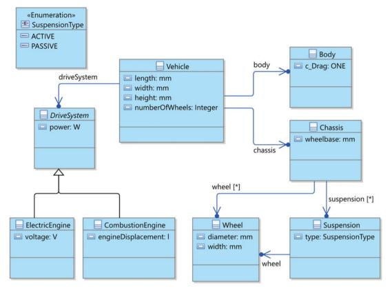
Fig. 2. Vocabulary for the design of a simple car model using the UML class diagram.
