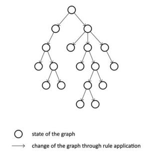
Fig. 5. Example of search in the search tree. Starting from an initial graph, many different solutions can be generated.
