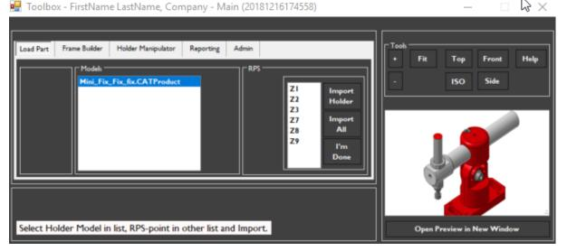
Figure 7. Demonstrator application Toolbox, ready to import holders to RPS-points on customer part.
