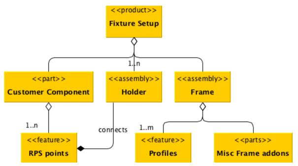
Figure 6. Product breakdown, following a Moka MML/UML-style structure notation.
