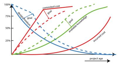
Figure 1. Expanded version of design process paradox; adapted from (Ullman, 2010) and (Verhagen et al., 2012).
