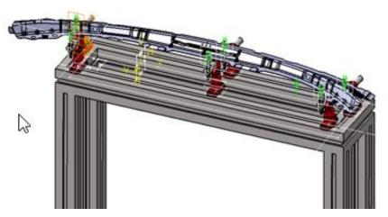
Figure 9. A final configured fixture.
