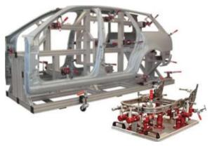
Figure 2. A fixture setup for control measuring.
