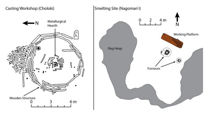
**Figure 6.** Plan of a secondary production workshop with casting debris (after Chavleishvili 1991, pl. 4) and a coppersmelting site (after Khakhutaishvili [1987] 2009, 90).
