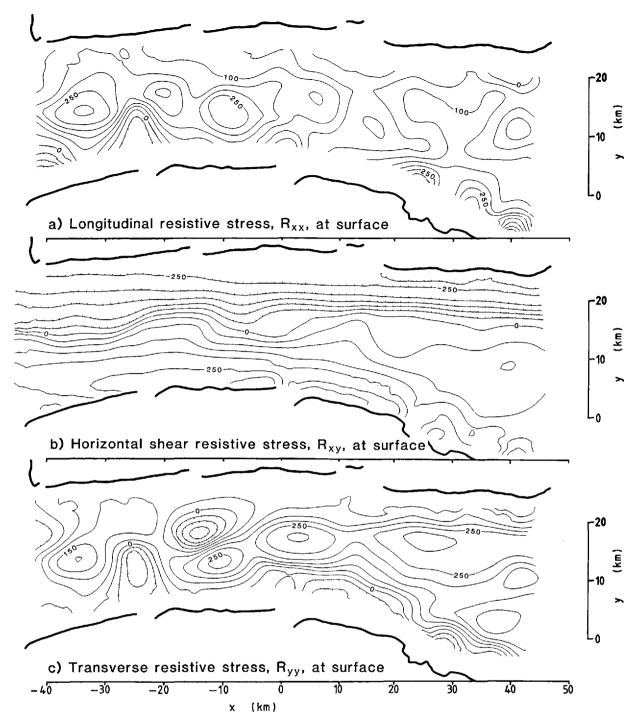
Fig. 4. Resistive-stress components at the surface, contour interval is 50 kPa.
