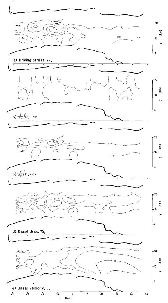
Fig. 10. Terms in the force budget in the y-direction and calculated  $\tau_{by}$ , and basal velocity,  $u_y$ . Like Figure 8 except that the more sophisticated calculation scheme is used.
