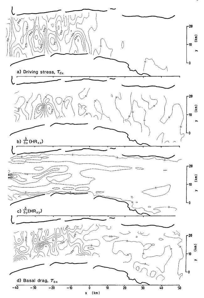
Fig. 7. Terms in force balance in the x-direction and calculated basal drag,  $\tau_{bx}$ , using the simplification that strain-rates are constant with depth, cross-valley thickness is constant, and the stiffness parameter, B, is constant. Contour interval is 50 kPa.
