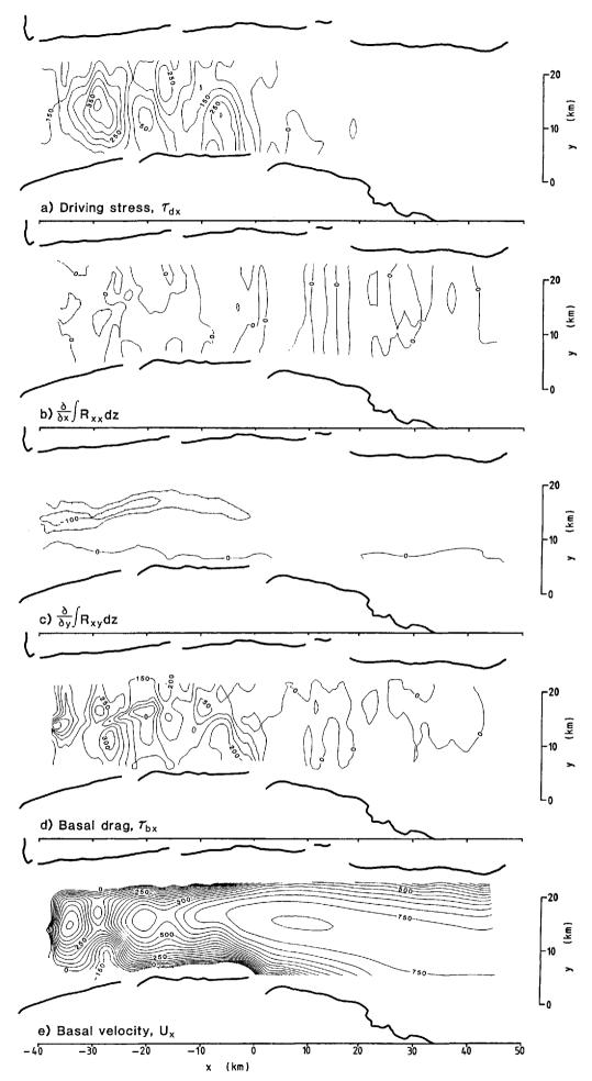
Fig. 9. Terms in the force budget in the x-direction and calculated basal drag,  $\tau_{bx}$ , and basal velocity,  $u_x$ . Like Figure 7 except that the stiffness parameter and velocity vary with depth and thickness is parabolic across the grounded part of the glacier. Calculations are performed for a more restricted area than for Figure 7 because funding ran out before we learned to adapt to irregular lateral boundaries.
