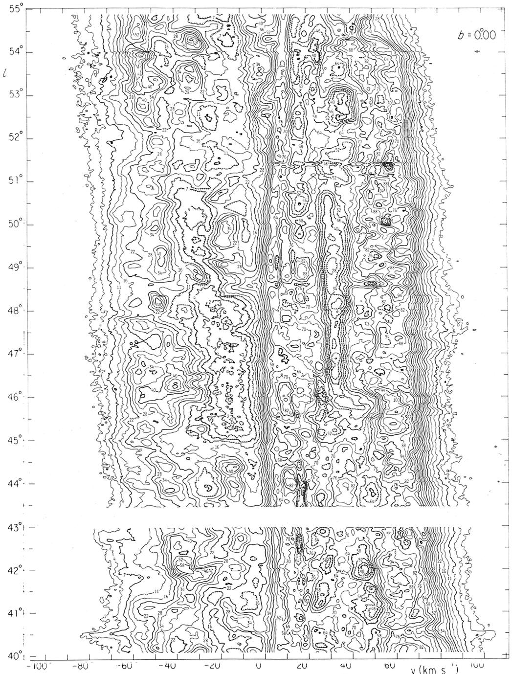
Figure 3.  $l$ - $v$  map of HI emission observed at  $b=0^\circ$  at the high angular resolution,  $3.2'$ , afforded by the Arecibo telescope (Baker and Burton, 1979). The map is peppered with small-angular-size intensity minima identified with self-absorption in cold clouds.
