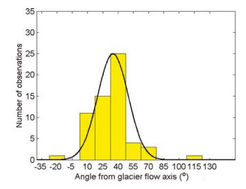
**Fig. 3.** Histogram of vertical fracture azimuth relative to glacier flow axis measured in boreholes on Bench Glacier. While the measured distribution shows some asymmetry, the overlain normal distribution, with standard deviation of  $\pm 15^{\circ}$ , provides a reasonable description of the variability in crack azimuth.
