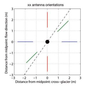
**Fig. 11.** Schematic that illustrates the GPR antenna polarizations at  $0^{\circ}$ ,  $45^{\circ}$  and  $90^{\circ}$  relative to the flow direction for the yy and xx polarizations, along with the estimated fracture direction. In yy polarization, the antennas are never aligned with the fracture direction, so the fast mode is always the first arrival observed from the bed.
