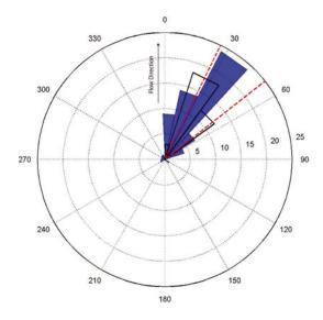
**Fig. 12.** Combined borehole-video (blue), seismic (black outline) and GPR estimates of crack azimuthal distribution (red dash). Angles are relative to the glacier flow direction. All three measurements are consistent and show a preferred orientation of basal crevasses that is oblique to the flow direction at  $\sim 30-45^{\circ}$ .
