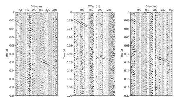
Fig. 4. Azimuth-averaged CMP supergathers, from three different locations in the 3-D seismic survey (see Fig. 2 for locations). The bed reflection arrives at  $\sim$ 90 ms at near offsets.
