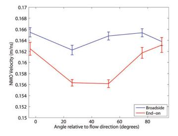
**Fig. 10.** Azimuthal variation in the GPR velocity is distinct and varies with polarization. Error bars show standard deviation in the velocity estimate from NMO analysis. Azimuthal variation is well above the estimated uncertainty of the velocity fit. The slow velocities of 0.156 m ns<sup>-1</sup> between 26° and 52° are measured with the antenna polarization aligned with fracture orientation measured in boreholes and estimated from seismic velocities.
