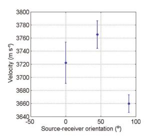
**Fig. 6.** Measured stacking velocities relative to glacier flow. These survey averaged velocities show azimuthal variation of 3.2%. Error bars show the standard deviation over all CMPs for each azimuth. Angles are azimuth relative to flow direction.
