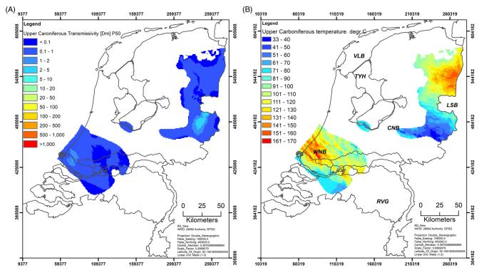
Fig. 14. Upper Carboniferous geothermal play maps. (A) The transmissivity map of the Upper Carboniferous reservoirs. (B) The average temperature of the combined Upper Carboniferous reservoirs. (Source: ThermoGis-v2.1, last accessed on 23 February 2019.) For structural elements abbreviations see Fig. 9.
