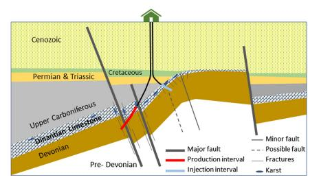
Production data shows that the wells are in a hydraulic connection trough, a complex permeability framework of fault, karst and fracture permeability.
