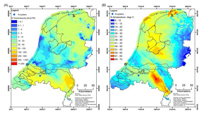
Fig. 7. Cenozoic geothermal play maps. (A) The transmissivity map of the Middle and Lower North Sea Group reservoirs. (B) The average temperature of the combined Middle and Lower North Sea Group reservoirs. Note the relatively low temperatures because of low burial depth. (Source: ThermoGis-v2.1, last accessed 23 February 2019.)
