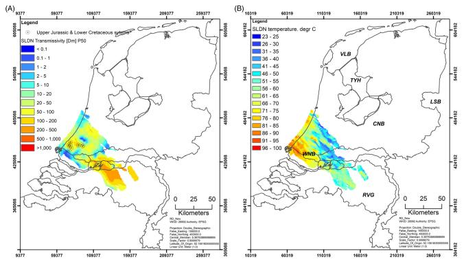
Fig. 10. Upper Jurassic, Nieuwerkerk Formation geothermal play maps. (A) The transmissivity map of the Nieuwerkerk Fm reservoirs. (B) The average temperature of the Nieuwerkerk Fm reservoirs. (Source: ThermoGis-v2.1, last accessed on 23 February 2019.) For structural elements abbreviations see Fig. 9. Note the Nieuwerkerk Fm is only present in the geological province West Netherlands Basin.
