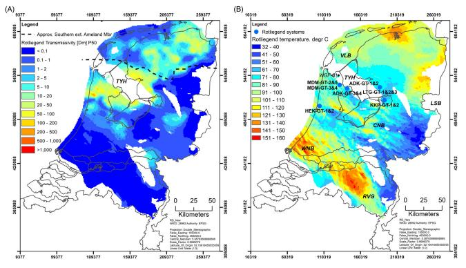
Fig. 12. Rotliegend geothermal play maps. (A) The transmissivity of the Rotliegend Slochteren Sandstone reservoirs. (B) The average temperature of the combined Rotliegend Slochteren reservoirs. (Source: ThermoGis-v2.1, last accessed on 23 February 2019.) For structural elements abbreviations see Fig. 9.
