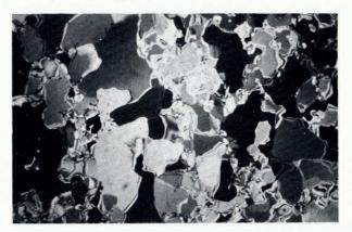
Fig. 14. Ice fabric from the April 1973 experiment; distilled-water ice deformed for 365 h.
