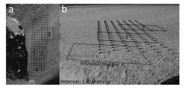
**Fig. 2.** The effects of perspective: (a) Landsat velocity determined from image pairs spanning 7–26 July 2002; (b) time-lapse photogrammetry derived velocities for the interval 22–23 July 2007. Arrows are (a) velocity and (b) pixels  $d^{-1}$  image displacements.
