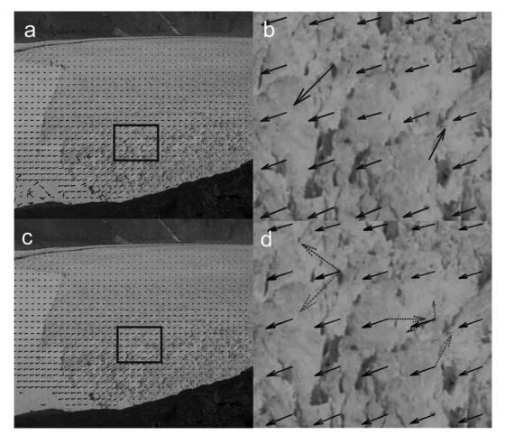
**Fig. 5.** Illustration of  $30 \times 30$  reference chip red-band displacement results from conventional matching (a, b) and from MIMC (c, d). Dashed arrows indicate outliers removed by the voting cell approach. Dashed arrows in (d) indicate cases where conventional matching fails.
