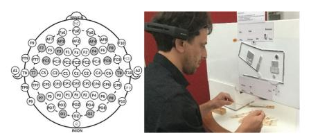
Figure 3. Emotiv Epoc+ electrodes highlighted in grey against the 10–10 I.S. layout and experiment setup using the headset.
