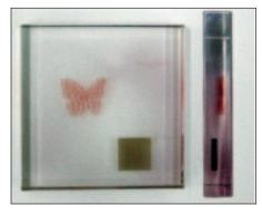
Figure. A butterfly created within a glass sample by femtosecond laser pulse excitation followed by oven annealing. The gray image has not been annealed. The size of the glass sample is  $50 \text{ mm} \times 50 \text{ mm} \times 8 \text{ mm}$ . The width of the butterfly is ~15 mm. Front and side views are presented.
