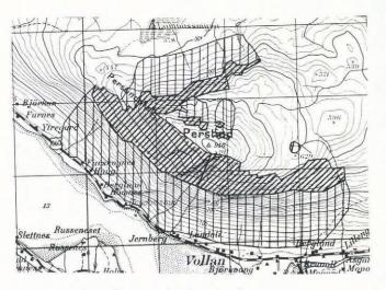
Fig. 6. Section of a completed avalanche map.
