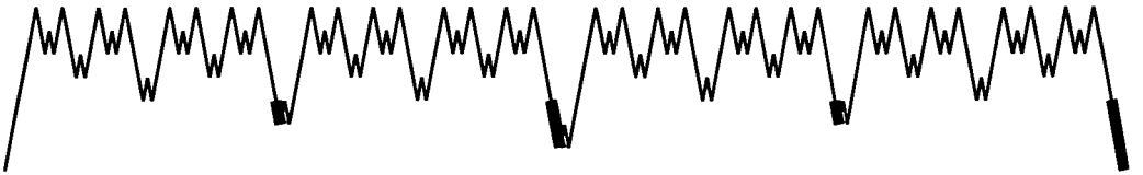
Fig. 9. Execution of T'(6) in a 16-line cache. Only the bold downticks (procedure returns) are read misses.
