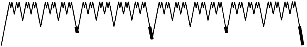
Fig. 8. Execution of T(7) in a 16-line cache. Every uptick (procedure call) is a write miss; only the bold downticks (procedure returns) are read misses.
