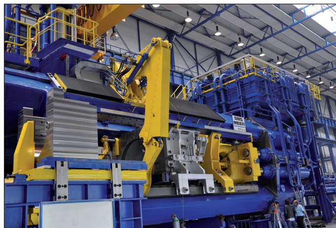
Profiles with lengths from 2 000 mm to 60 000 mm and diameters up to 700 mm will be produced. Photo courtesy of SMS Meer
