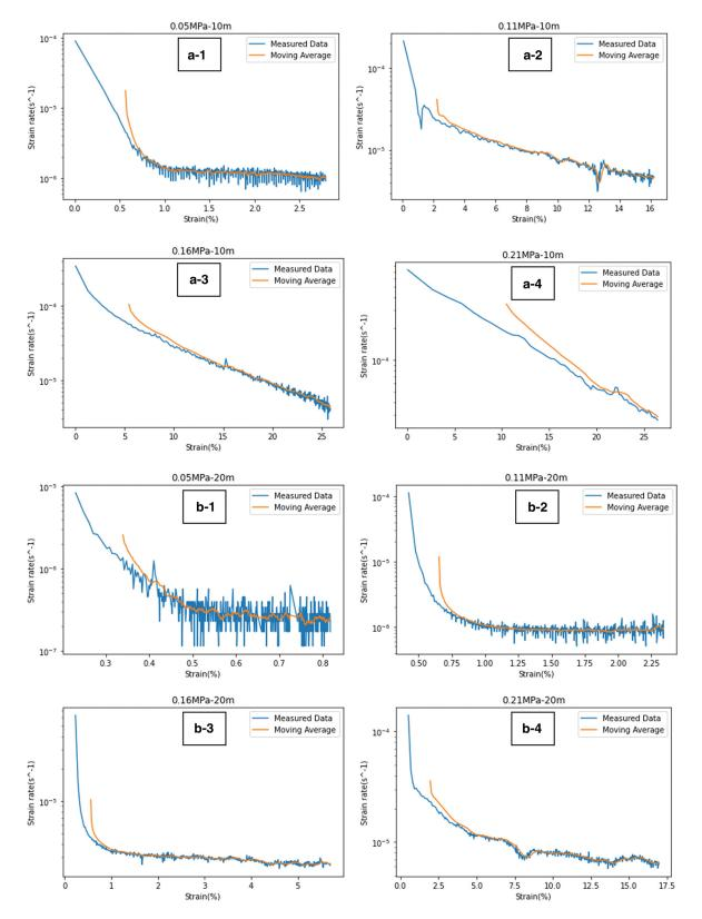
**Fig. 6.** Graphs of log strain rate versus strain for 10 m (a), 20 m (b), 30 m (c), 40 m (d), 50 m (e), 60 m (f), 70 m (g) and 80 m (h) firn samples, where the sub-graphs for the different applied stresses indicated at the same depth are labeled sequentially as 1, 2, 3, etc. The blue lines represent the discrete strain rates, which are calculated by extracting the strain data hourly, while the orange lines represent the moving average by 15 moving windows with respect to the strain.
