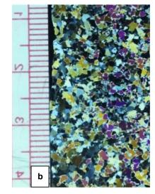
**Fig. 4.** Optical photographs of thin sections before (a) and after creep (7.6% strain) (b) for 60 m sample at a load of 0.43 MPa.
