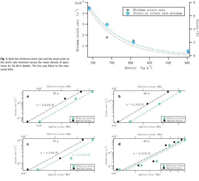
**Fig. 8.** Log strain rate versus both log applied stress and log effective stress for the 50 m (a), 60 m (b), 70 m (c) and 80 m (d) firn core at stresses excluding data from the 0.05 MPa specimens at each depth, where a minimum strain rate is observed. The stress exponents indicated were obtained for both the applied stress (black color) and the effective stress (green color). The broken line denotes a fitted line from measured data.
