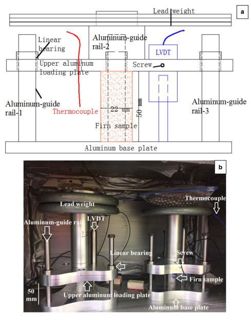
Fig. 1. 2-D schematic (a) and photograph (b) of home-built compressive creep jigs. See text for details.
