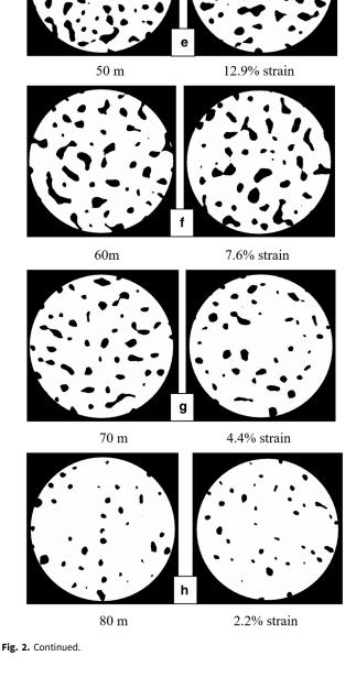
**Fig. 2.** Micro-CT 2-D reconstructions of the creep specimens before and after creep testing from 10 m (0.21 MPa) (a), 20 m (0.21 MPa) (b), 30 m (0.21 MPa) (c), 40 m (0.43 MPa) (d), 50 m (0.43 MPa) (e), 60 m (0.43 MPa) (f), 70 m (0.43 MPa) (g) and 80 m (0.43 MPa) (h). The diameter of cross-section is equal to 12.8 mm. The pores are shown in black and the ice in white.
