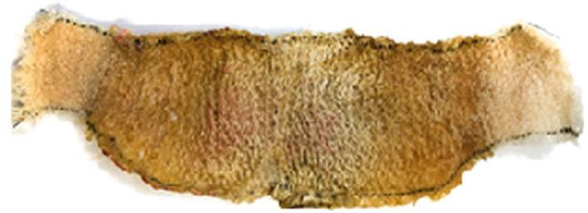
**Figure 1.** Agitated culture of Bacterial Cellulose pellicle grown on Pemetex knit textile sample.
